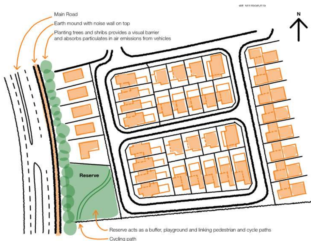
Figure 39 – Example of low density housing adjacent to an expressway with a noise barrier and separation distance to reduce noise emissions (Source: DPTI 2012)
