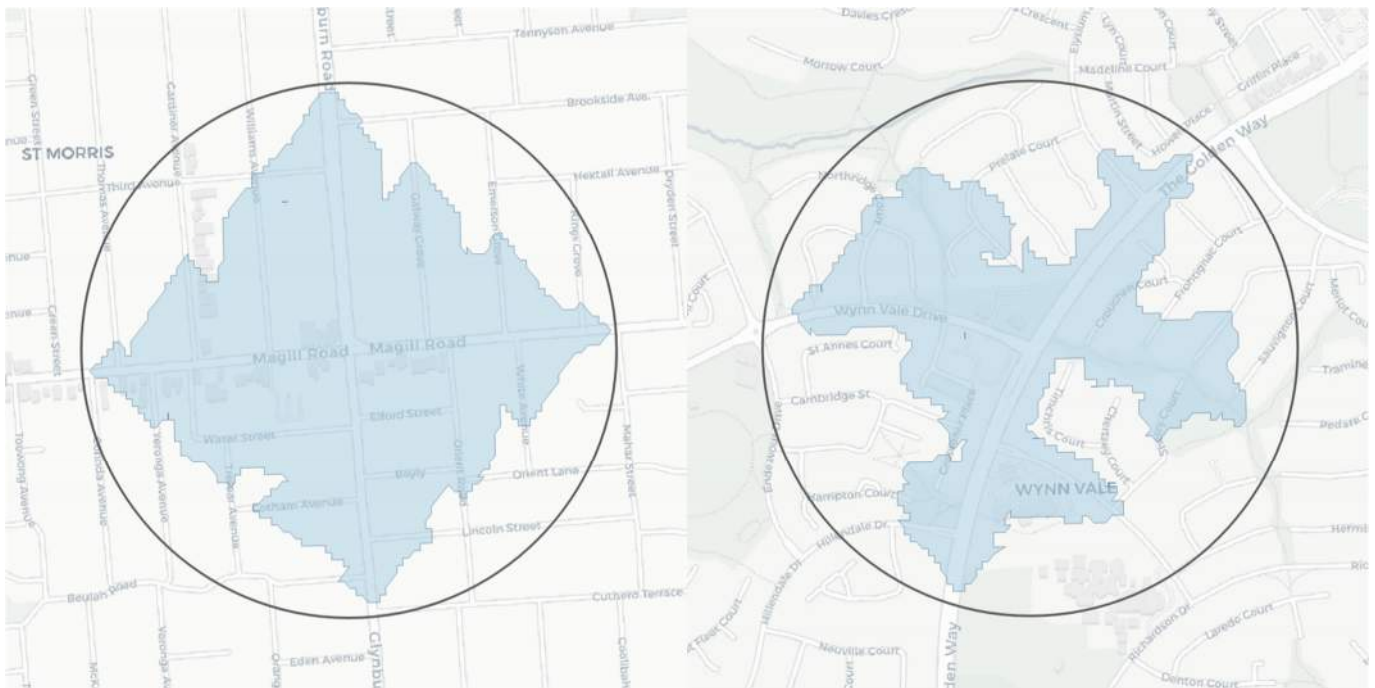
Figure 26: Impact of road network topology on area reachable within a 5 minute walk. Connective grid type network on the left and disconnected, hierarchical cul-de-sac type network on the right.
