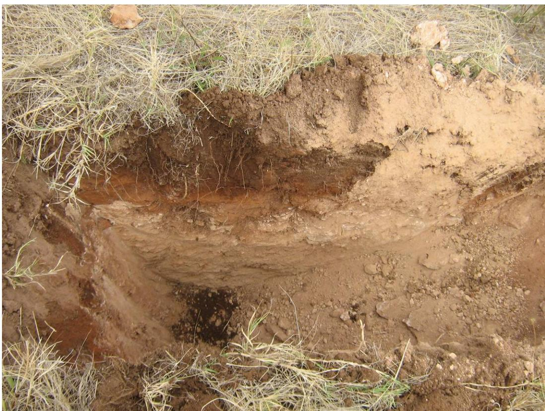
**Photo 1      Test-pit 03, indicative of soil profile encountered in northern portion of the site**
