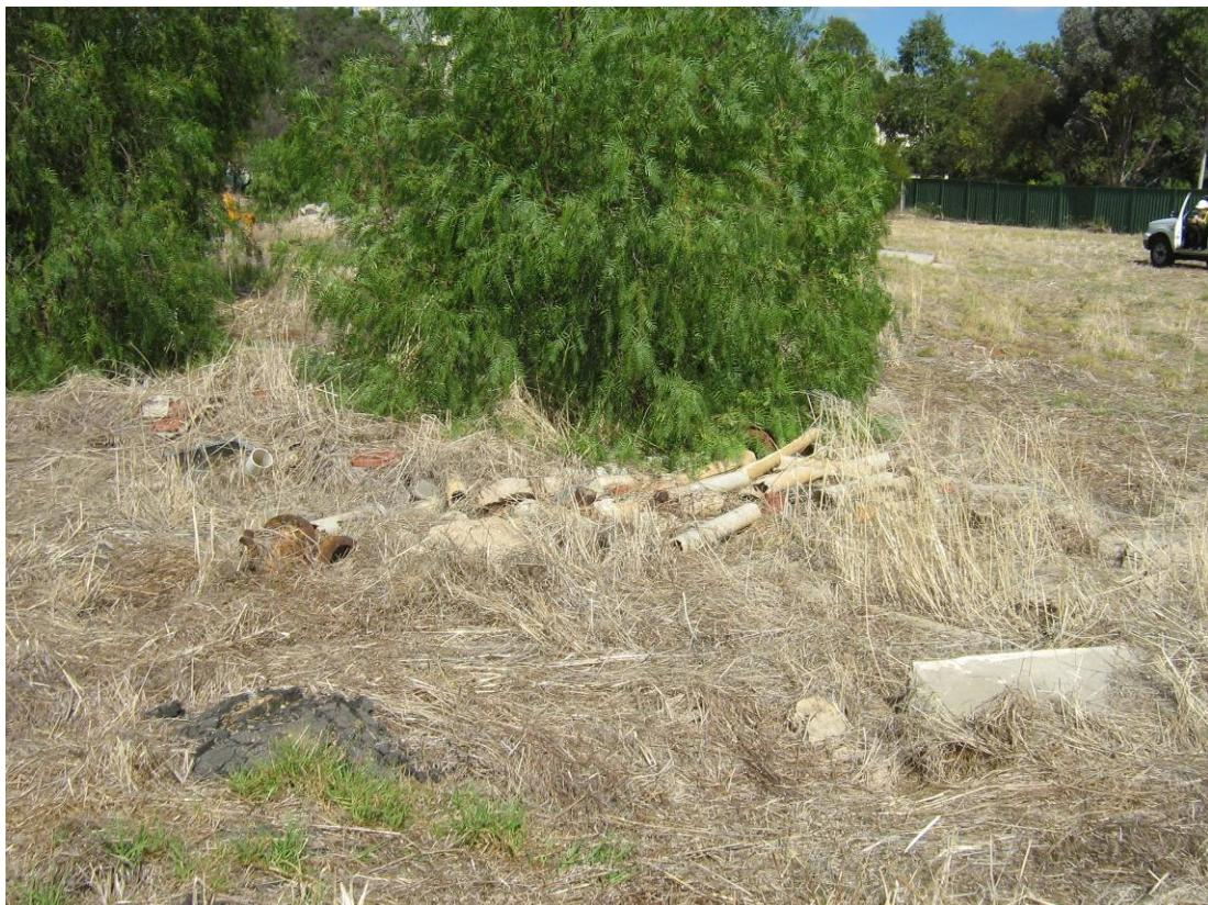
**Photo 9 Asphalt and asbestos cement piping disposed in the vicinity of the former Ward 3 building**
