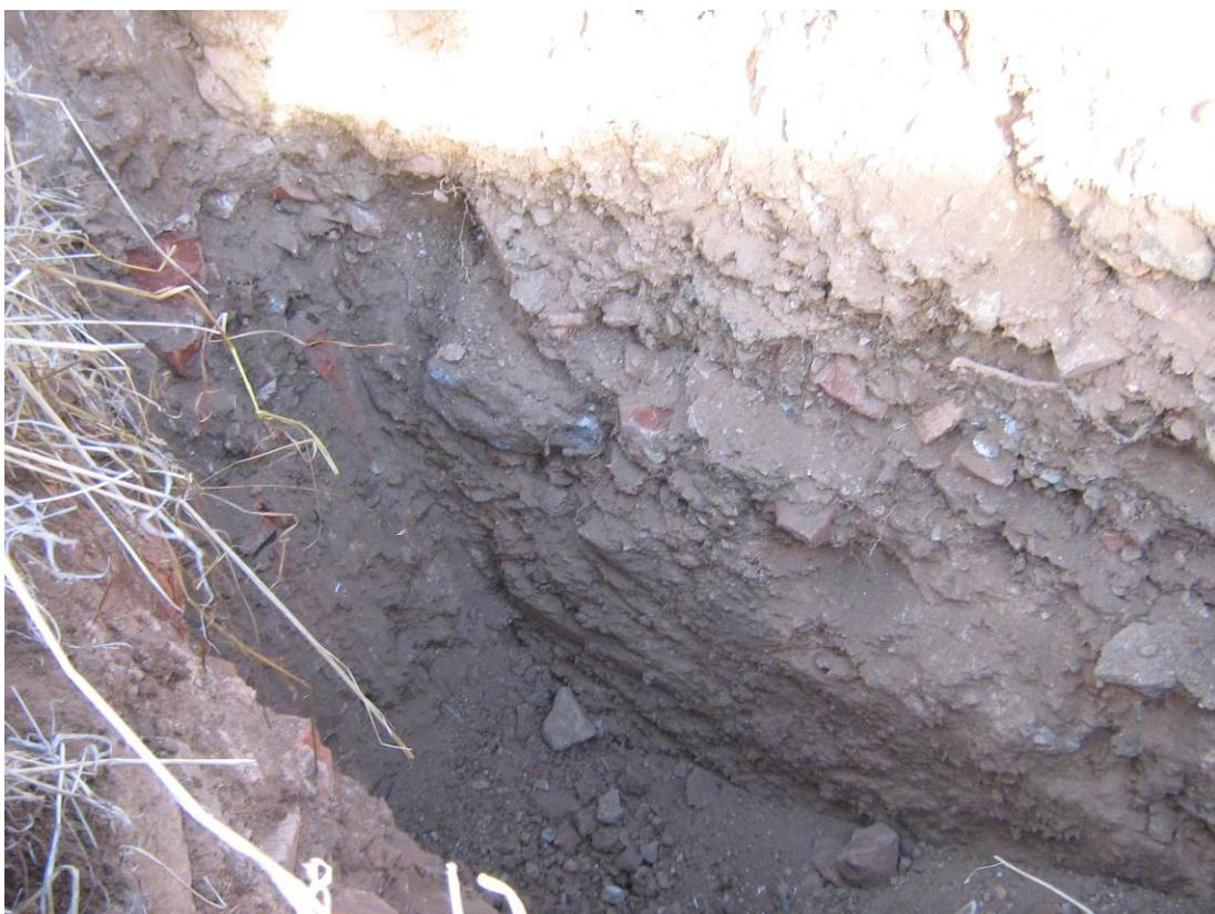
**Photo 3 Delineation-pit 18 showing buried building demolition material**
