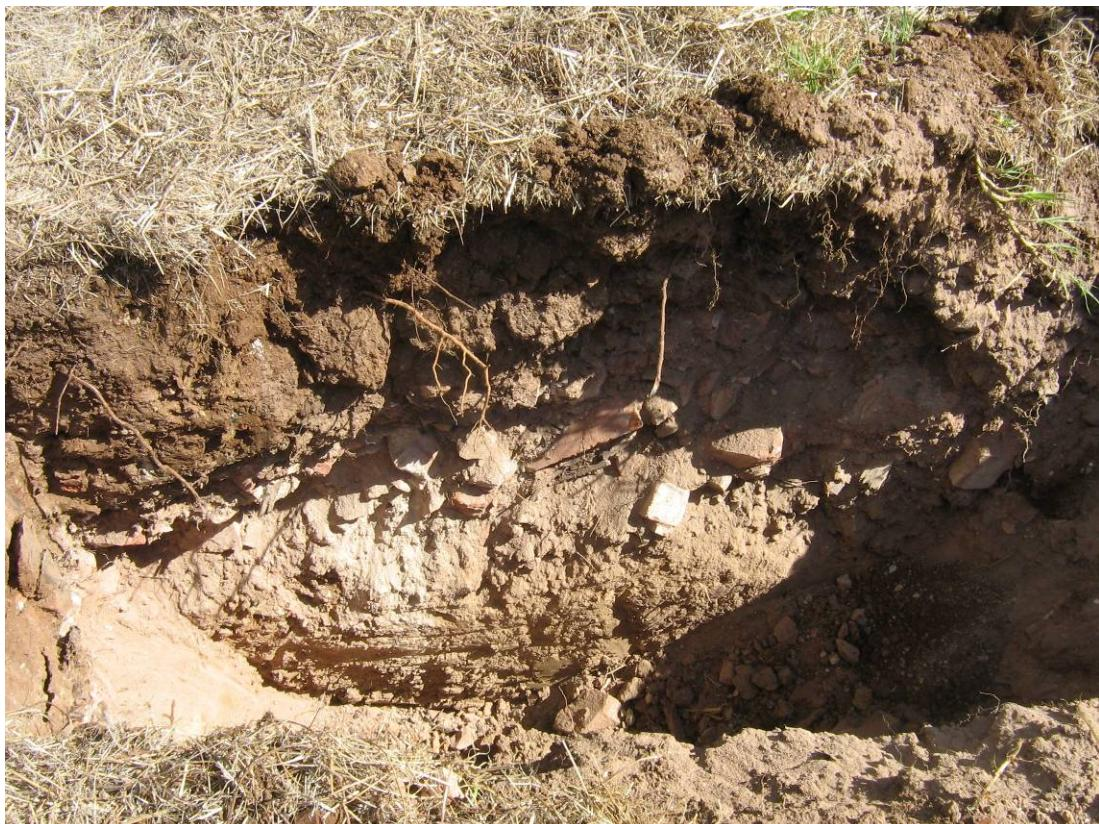
**Photo 5      Test-pit 28 located in the vicinity of the former Ward 3 building, showing buried building demolition material**
