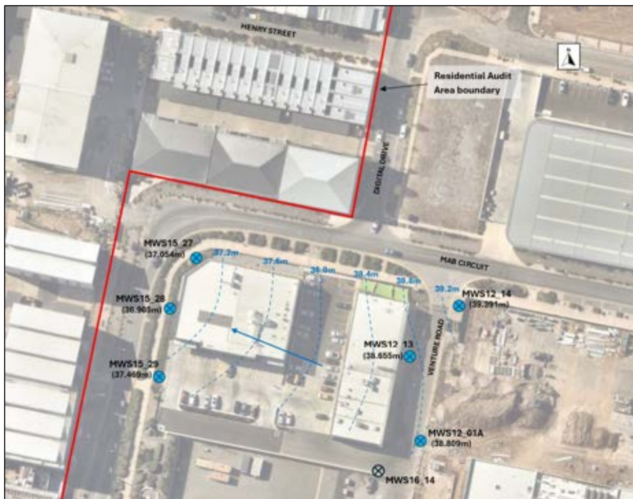
Figure 6: Groundwater levels (m AHD) and inferred flow direction
